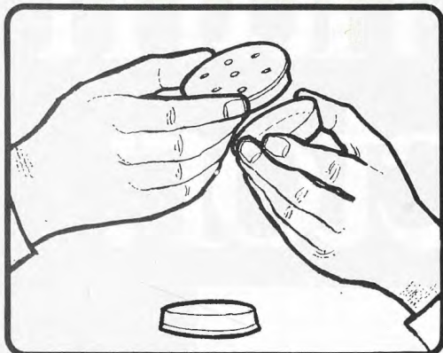
1 Template fits accurately into plate.
